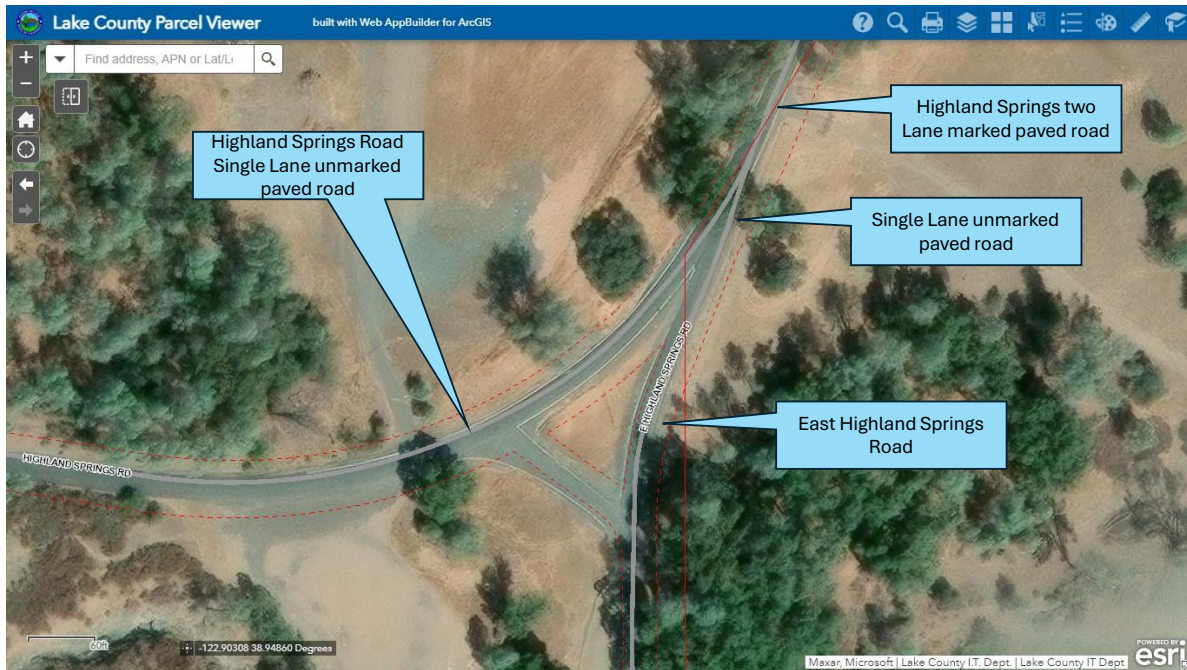
Figure C5: Aerial view of Highland Springs Road transition from two to one-lane
