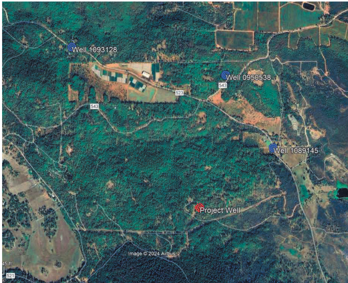
Figure 2. Location of wells with reported first encountered water and static water levels.
